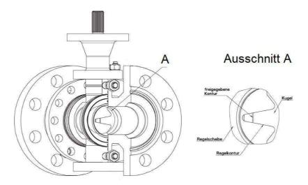
The 90° turn by the ball over the control disc(s) opens the control diameter and thus regulates the control function.
